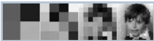
◀ Increasing the number of electrodes in contact with the retina increases the image quality; these simulated images show the expected difference between four, 16, 64 and 1,500 electrodes
