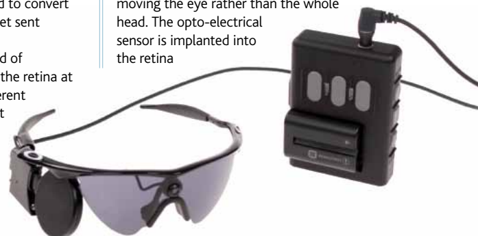
▲ The Second Sight Argus II Retinal Prosthesis System uses a video camera built into a pair of sunglasses to transmit images wirelessly to the implant in the retina
