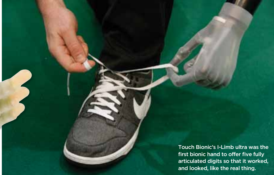
▲ Touch Bionic's I-Limb Ultra was the first bionic hand to offer five fully articulated digits, so it worked – and looked – like the real thing
